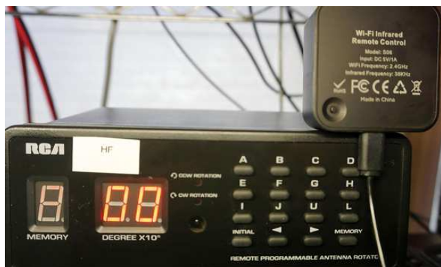
Figure 2 — The Wi-Fi infrared hub shown atop the RCA VH226E controller. [Tommy Walls, KC4ZZE, photo]
