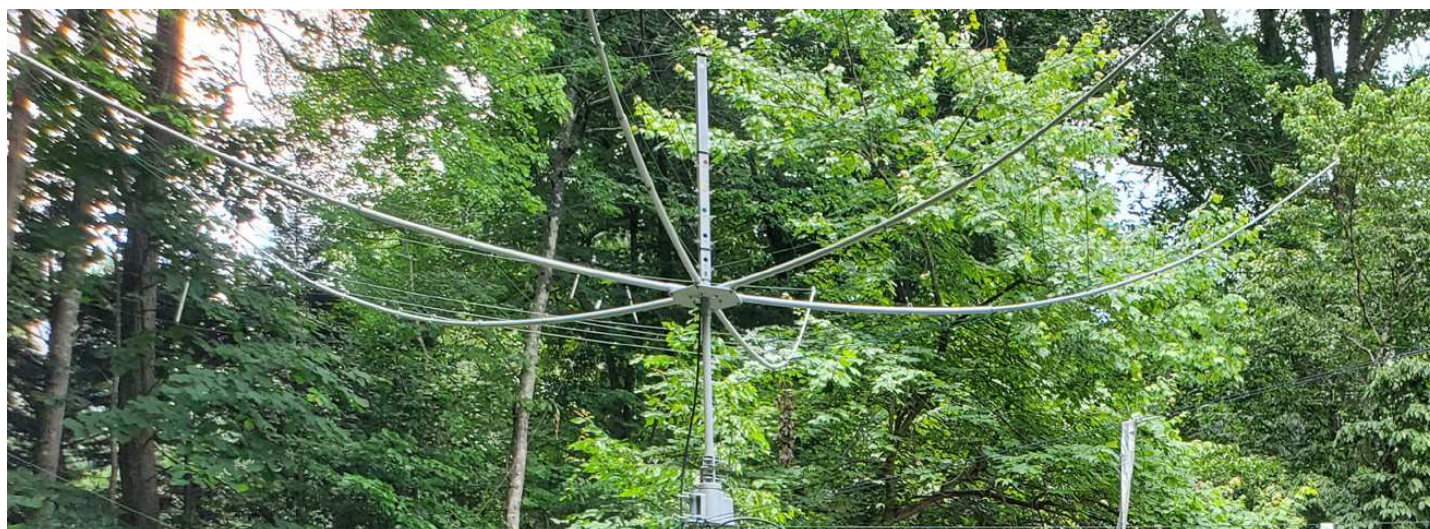
Figure 1 — The hexbeam antenna and RCA VH226E rotator. [Tommy Walls, KC4ZZE, photo]
